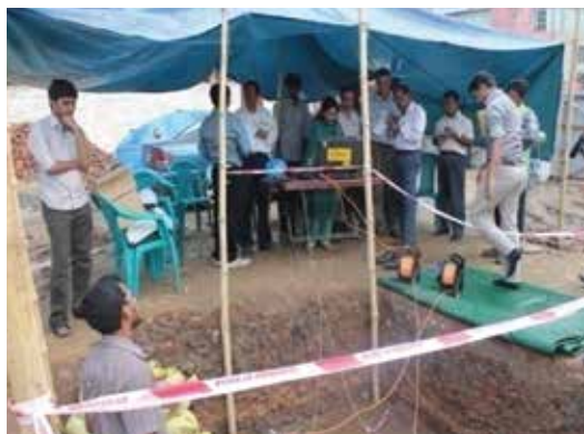
Screw Plate Load and Cross-hole Test on test pil (Dr. Sarah Tahsin Noor)
