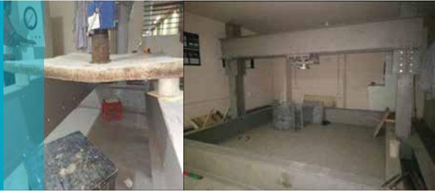
RC Slab Testing by Loading Frame
